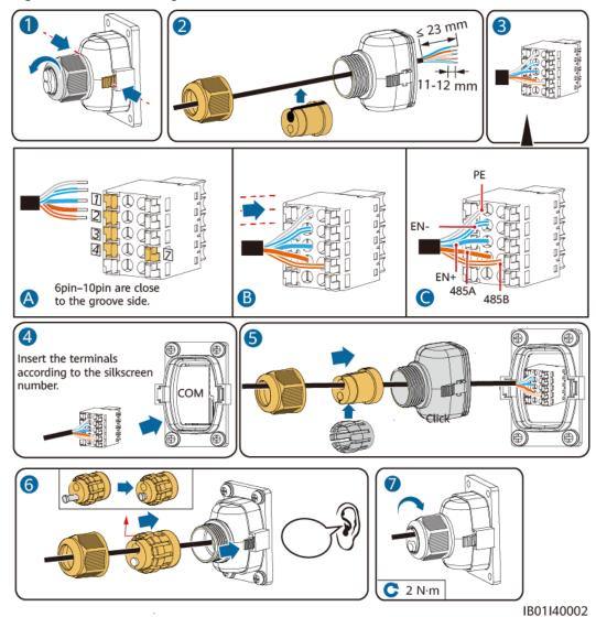
Figure 5-14 Connecting inverter terminals
