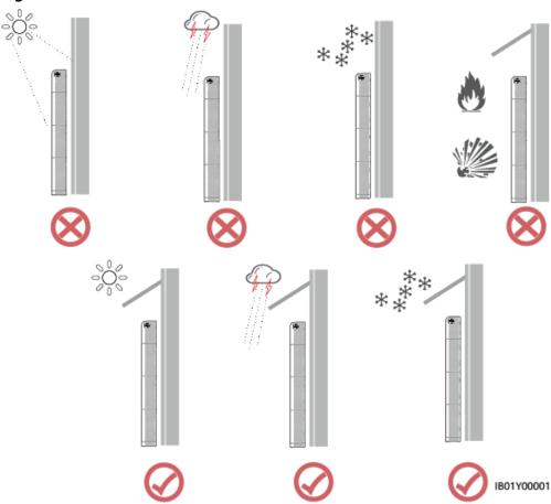
Figure 1-1 Installation environment
