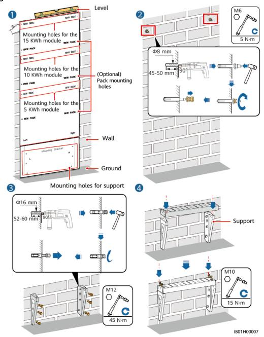
Figure 4-8 Wall-mounted installation
