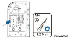
**Step 3** Lift the fuse box opening, remove the fuse, insert a new fuse into the slot, and close the fuse box. If you hear a click sound and the bulge on the side is inside the box, the fuse box is properly installed.
