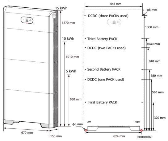
Figure 4-2 Floor-mounted installation dimensions
