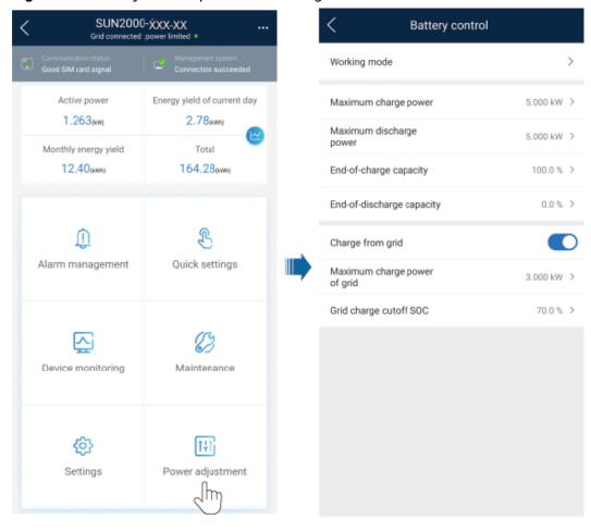
Figure 6-6 Battery control parameter setting
