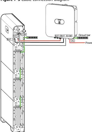
Figure 7-3 Cable connection diagram
