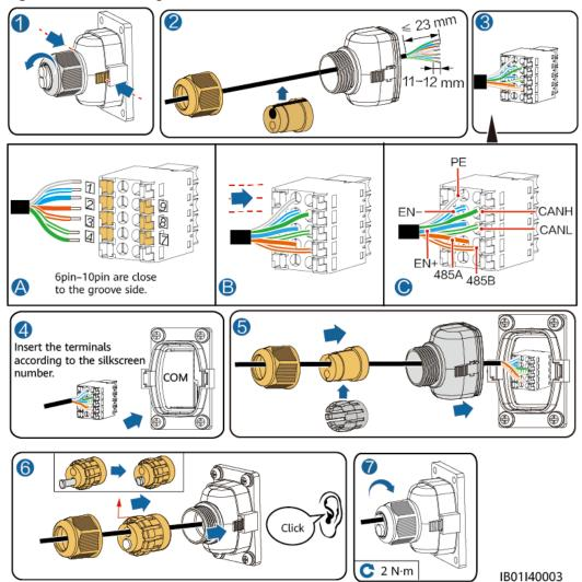
Figure 5-17 Cascading communication terminal
