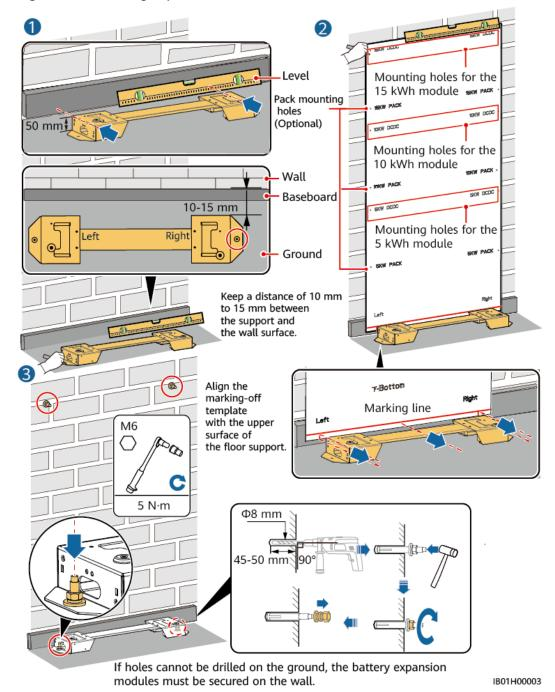
Figure 4-4 Installing expansion bolts
