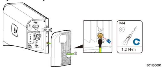
It is recommended that silica gel or paint be used around the ground terminal after the PE cable is connected.
