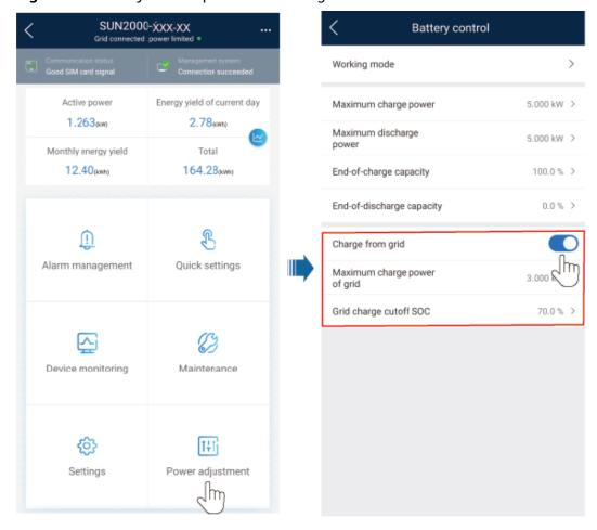
Figure 3-7 Battery control parameter setting
