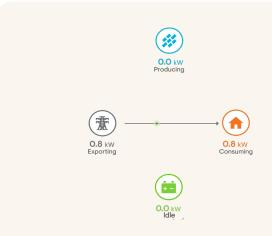
The battery has reached its minimum reserve capacity and can no longer be used to power the home, so energy is being imported from the grid.
