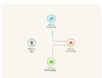
Solar production and battery discharge are powering the home.
